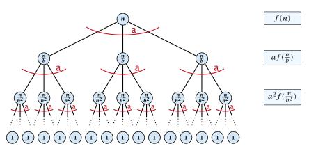
The running time of a recursive algorithm can be visualized by a recursion tree:
