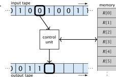
Note that in the picture on the right the tapes are one-directional, and that a READ- or WRITE-operation always advances its tape.
