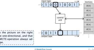
Note that in the picture on the right the tapes are one-directional, and that a READ- or WRITE-operation always advances its tape.
