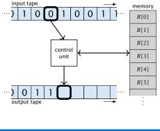
Note that in the picture on the right the tapes are one-directional, and that a READ- or WRITE-operation always advances its tape.
